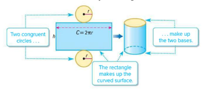
In the diagram above, the length of the rectangle is the same as the circumference of the circle,  $2\pi r$ . Also, the width of the rectangle is the same as the height of the cylinder.
